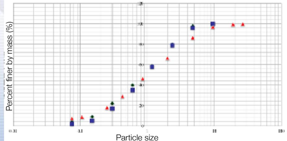
Large particle distribution contributes to the good compaction characteristics of ARC-Sand
